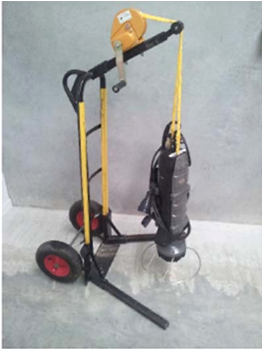
Figure 4: Example pump lifting device
