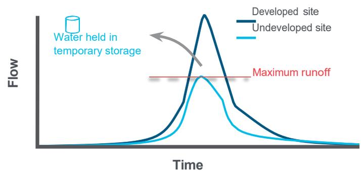
**3** This method can bring peak flow rates during significant rainfall events to a level much closer to that of undeveloped sites. Our goal is to meet the definition of hydraulic neutrality.
