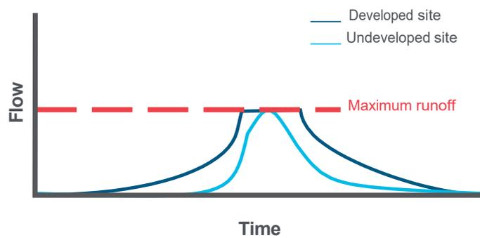
**We define hydraulic neutrality as capturing post-development peak runoff so that it does not exceed the pre-development peak flow rate.**
