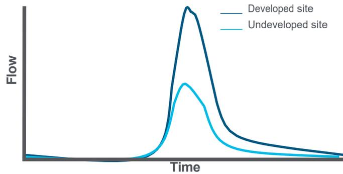
**2** The increased difference in peak flow can be captured and held in temporary storage devices to be used in other applications or slowly released back into the stormwater network.
