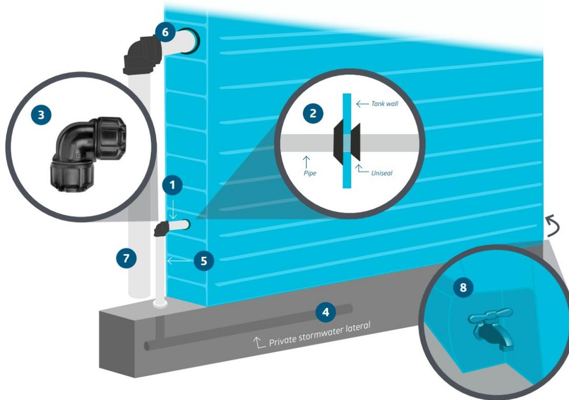
1. A short 20mm diameter pipe is inserted into the tank end at the required height (see Table 1-2). The pipe is held secure to the tank using a Uniseal or similar product. For a 20mm diameter pipe it is recommended to use a 31.7mm holesaw size to drill your outlet.
