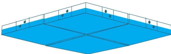
This solution is for modular tanks with a capacity of 350 litres – additional tanks are added to build up the storage capacity to the volume required to achieve hydraulic neutrality. The tanks lock together using connector pipes that allow stormwater to flow between tanks. Water will flow out of the tanks via an orifice and outlet pipe that will be connected to the stormwater network.
