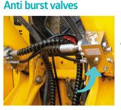
Fitted to all excavators 7T and above
