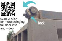
Must be fully locked out when working for WW or fully complies with FH swinging tail door standard. There are many different lock options
