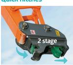
Hitches must be 2 stage or pinned type
