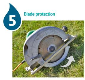
• Ensure the retractable blade guard has sprung back to cover the exposed blade before placing the skill saw down
