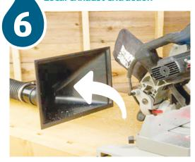
Exhaust extraction systems should be considered for established workshops and long term projects. These must be designed correctly as there is a risk of explosion from some dusts
