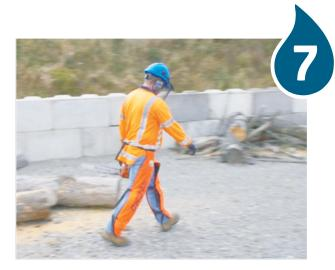
If walking a long distance turn the saw off and for short distances, brake the blade
