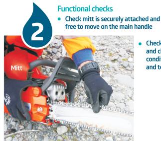
**Check bar** and chain condition and tension
