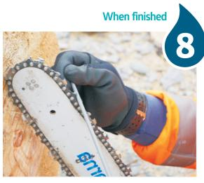
Service and clean the chainsaw and apply bar guard prior to storage
