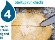
Upon startup, apply revs, check the chain brake is working and confirm bar lube application
