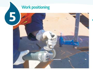
Ensure that what is being cut is secured against movement
